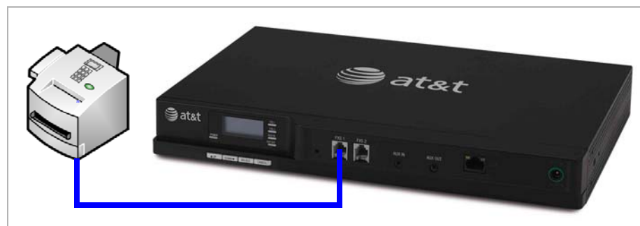
Figure 3. Fax Machine Connected to FXS Port
